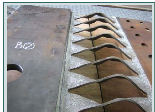
After a shaking test, a (formerly flat) steel fuse shows the deformation caused by the energy it dissipated during shaking. The fuses are designed to absorb damage and are easily replaced after an earthquake. Image Credit: Tsuyoshi Hikino, National Research Institute for Earth Science and Disaster Prevention, Japan
