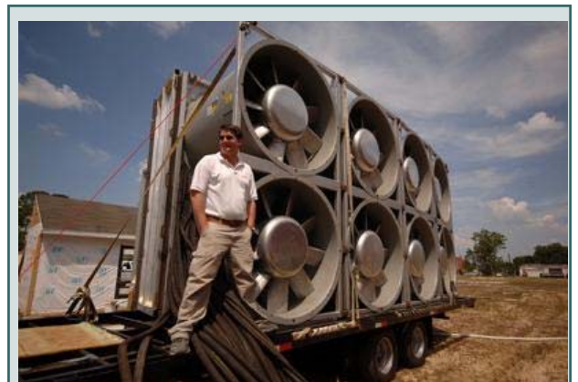
University of Florida wind engineering researcher Forrest Masters stands on a newly completed, fully portable hurricane wind simulator.
