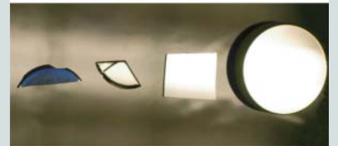
Layers of silica nanorods look like shag carpet (top) when viewed with a scanning electron microscope. When coated on a surface (bottom), the new anti-reflective material looks dark (left) in contrast to other anti-reflective coatings.
