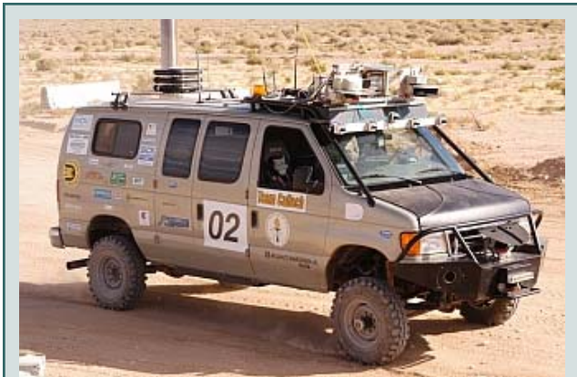
The autonomous van "Alice" is Caltech's competitor for the Defense Advanced Research Projects Agency Grand Challenge, a race that features autonomous ground vehicles. The challenge demonstrates how the U.S. military safely conducts supply missions in cities with heavy traffic. Credit: Caltech
